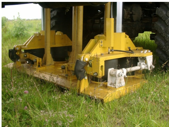
Vibrator Baseplate, Down Position
